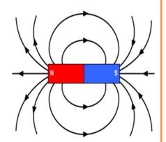
A permanent magnet produces its own magnetic field that cannot be turned off.
